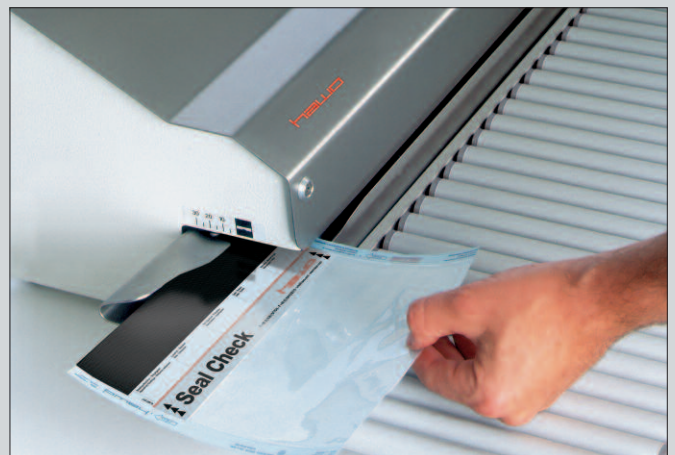
Sealing seam testing with hawotest Seal Check
